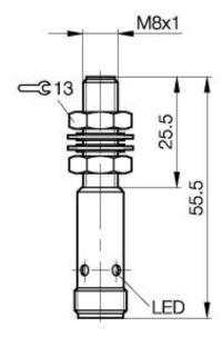
**Inductive Sensors** BES 516-324-G-E5-C-S 49 M8x1 x 45 normally-open Sn=2mm shielded
